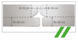
The cutting pattern also applies to the formation of skylight corners, etc.
