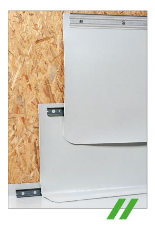
Alternatively, the membrane can also be adhered to the entire surface with KÖSTER Contact Adhesive. The contact adhesive must be applied over the entire surface both to the component and to the membrane to be bonded. The adhesive must dry briefly, this can be checked with a finger test. The glue must no longer pull threads.
